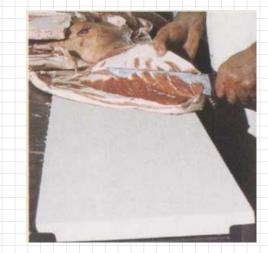
**UHMW-PE** is a widely acceptable food grade plastic. It is hygienic, resistant to acids & alkalis, also does not absorb any moisture. Widely used in Hotel industry as chopping boards & also where it has to be used in direct contact with the food.
